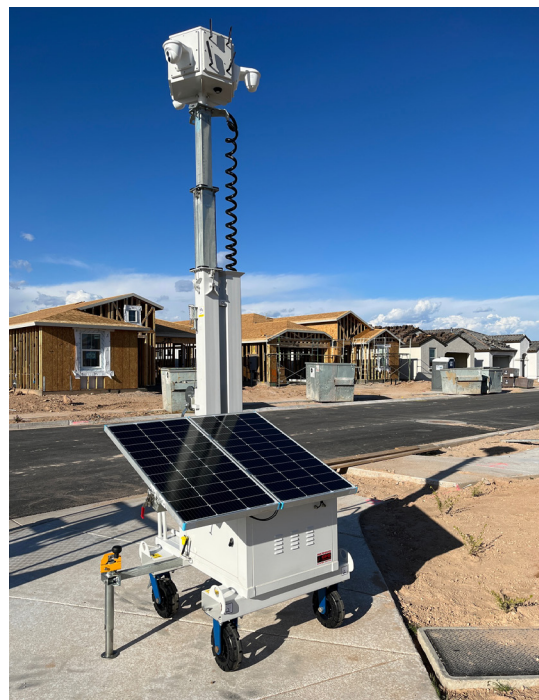
Carts and trailers rapidly deployable by a single person in less than 5 minutes
